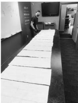
A pleated media filter, like those manufactured by Aprilaire or Amana, provides less restriction to airflow. This is accomplished by increasing the amount of surface area that the air must pass through by using many pleats or folds. When fully stretched out, an Aprilaire 16 x 20 filter has about 19 feet of media as shown in photo to the left.
